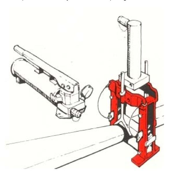
When repairs are completed, re-install the hydraulics and apply only enough pressure to loosen the wedge locks. Remove the wedge locks and slowly release the pressure. A slow reduction of pressure is as important as a slow squeeze rate.
