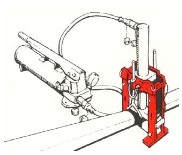
The pipe-choke may be rotated 90° and pressure re-applied to re-round the pipe. Inspect the squeezed area. Report any damage immediately. Mark the squeezed area.
