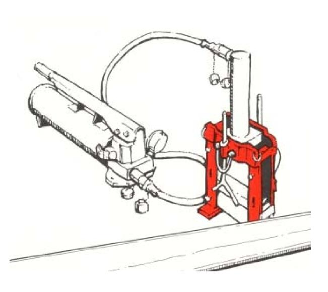
Place the pipe-choke tool over the area of pipe to be squeezed. Center the machine on the pipe. Make sure the correct stops are in place and the tool is grounded. (Follow your company's squeeze-off procedures exactly.)
