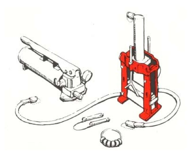
Assemble the squeeze unit. Visually inspect your equipment and test it to ensure proper operation. Pipe-choke tools should be maintained in good working order for emergency use. Examine the hydraulic hose(s) for kinks or nicks before each use.
