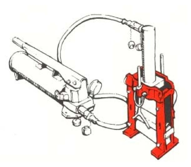
Check the pipe area that will be squeezed. **DO NOT** attempt to squeeze an area of pipe that has been squeezed-off previously. Make sure that you have enough work space for the pipe-choke and for the repair work.
