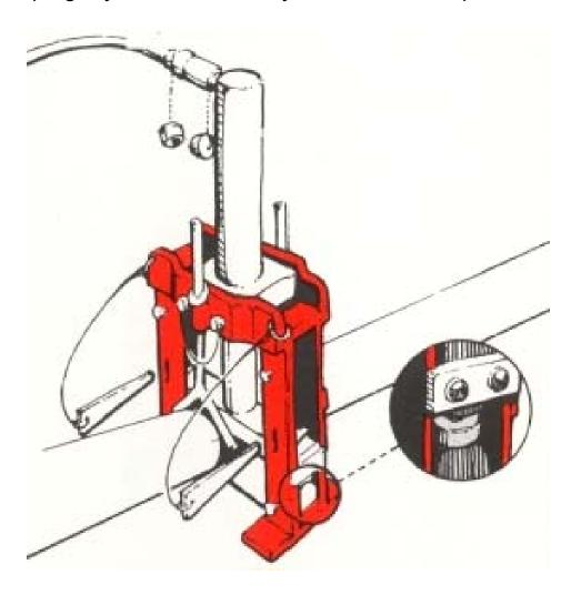
Remove the hydraulics. The wedge locks will keep the pipe squeezed-off and will help to eliminate any release or tampering.
