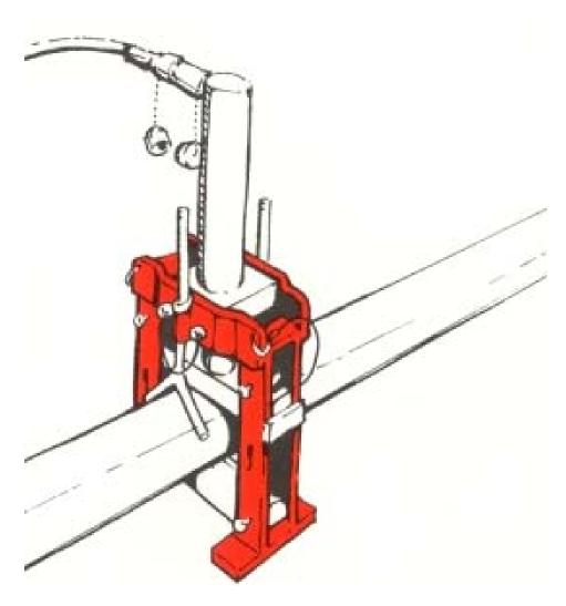
Begin to apply pressure until the squeeze bars seat on the squeeze stops. A slow, uniform rate of pressure will lessen possible damage to the pipe. Place the mechanical back-up lock wedges in position and tap lightly to lock. Visually examine the squeeze-off.
